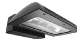
LED V-line Wall pack are designed with a high quality die cast housing. Durable chip and fade resistant powder coat finish. Efficient design separates the driver from the LED to minimize heat, air cooling design of aerodynamic and modern appearance. Adjustable head for precise aiming.
